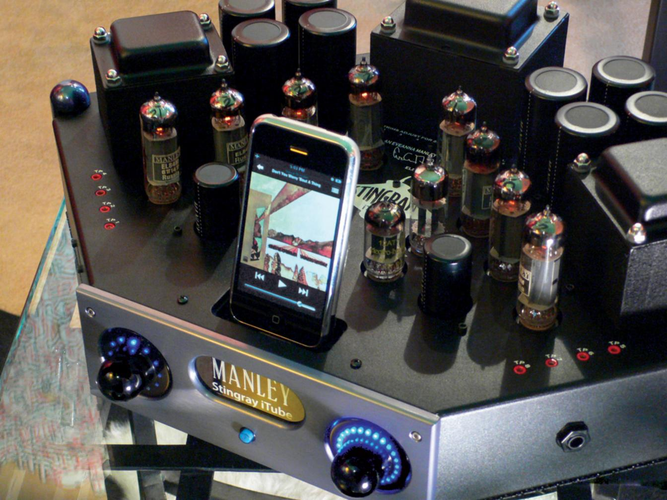
An iPod dock has been integrated into the Stingray iTube as the 4th input source. The Manley iTube has been certified by Apple and officially sanctioned as a "Made for iPod" product. The Stingray's Remote Control commands the iPod PLAY/PAUSE and TRACK FORWARD/BACK controls.
